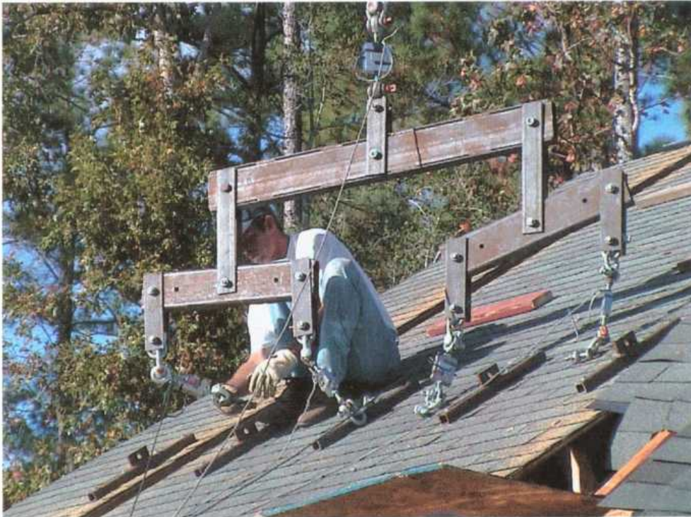
Figure 4. Loading Tree and Load Cells Used in Uplift Tests
